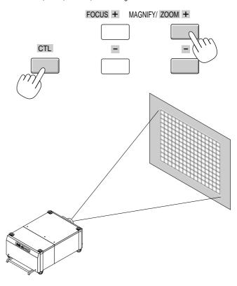
(3) Press and hold the CTL button and press the FOCUS + or - button to obtain the best focus optically. You can also adjust the focus by using the FOCUS + or - button on the projector cabinet.
